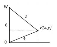
Show that  $s^2 = 52 - 12y$  and hence determine the rate at which x is decreasing at the instant that y is increasing at a rate of 10 cm/s.
